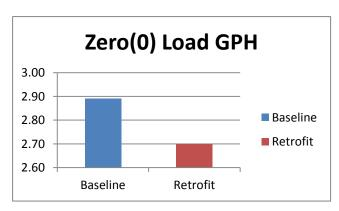
The engine was started and brought up to normal operating temperature prior to commencing the test for baseline and retrofit data collection. Upon starting of the pre-programmed script which controlled the load applied to the gen-set, data collection began.
