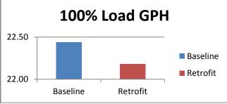
The above charts illustrate a comparison of the average of the 20 readings taken at each load point. There was never more than one-tenth (0.10) gph range in any set of data. At least 18 of the 20 readings were exactly the same demonstrating the accuracy of the fuel meters used.
