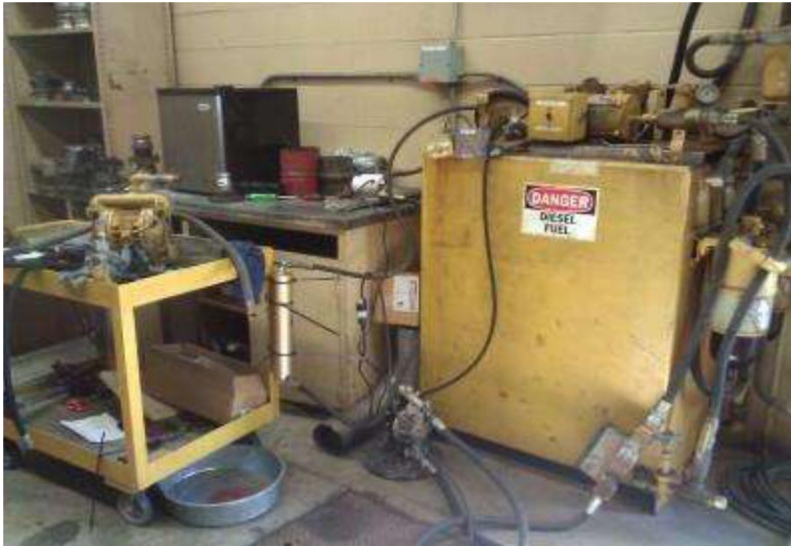
200 gallon day-tank used to supply ULSD#2 for test. Close-up of AIC-6008 fuel flow meter Fuel Measurement Results
